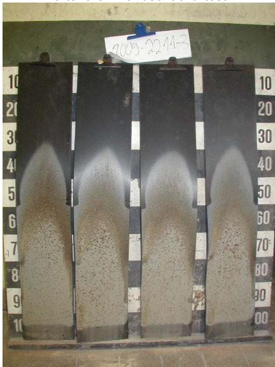
Appearance of sample C after the "Brandschacht" test
